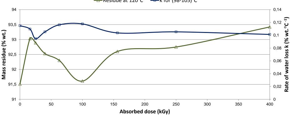
Dependence of residual mass at 120°C and rate of water loss in degreased dry wool (WD) on absorbed dose within range of (98-105)°C on absorbed dose
