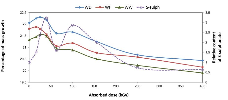
Comparison of humidity uptake for all wool samples depending on absorbed dose and related to content of S-sulphonate in the degreased dry wool (WD)
